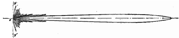
Figure 4—Distribution of Field in a Horizontal Plane of an Antenna Array Having Both Radiators and Reflectors.
